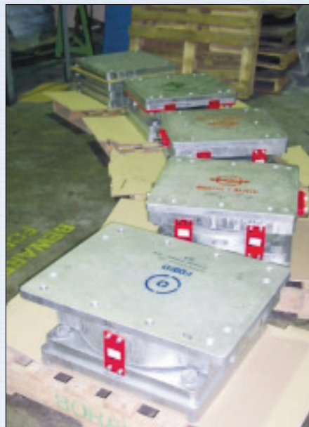
Ready for shipment – 5,000kN Fixed, Free Float and Guide/Slide Pot Bearings.
